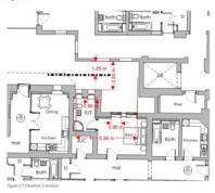
The plane of reference for this analysis is taken to the national boundary between the neighbouring building parallel to the elevation. The unprotected area of this compartment elevation is approximately (0.6x2.7 + 0.6x2.7 + 0.9x2.7 + 0
